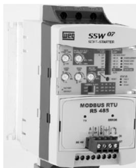
When the interface RS-485 is used, the master can control several drives connected to the same bus. The Modbus-RTU protocol allows the connection of up to 247 slaves (1 for each address), provided also signal repeaters are used along the bus. This interface has a good noise immunity allowing cable lengths up to 1000 m.
