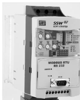
This interface enables the connection of the master to a Soft-Starter SSW-07/SSW-08 (point-to-point) at distances up to 10m. For the communication with the master you must use one wire for the transmission (TX), one wire for the reception (RX) and one wire for the reference (PE).
